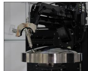
The world's most versatile, non-contact 3D form measurement platform for advanced large diameter optical surfaces
