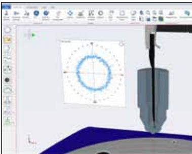
A powerful utility that enables online and offline programming around a CAD model. Features include a stylus tip “flight path” enabling collision detection.
