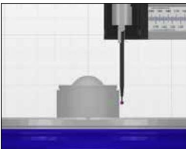
A simple approach to gauge calibration that literally takes seconds to do. Utilising the instrument high precision scales this procedure calibrates both the gauge gain and crutch angle position in a single user guided operation.
