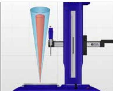
The smaller the coning error of any instrument the more reliable the results. In fact, coning error is the single biggest source of error when measuring cylindricity, parallelism and roundness of tall components.
