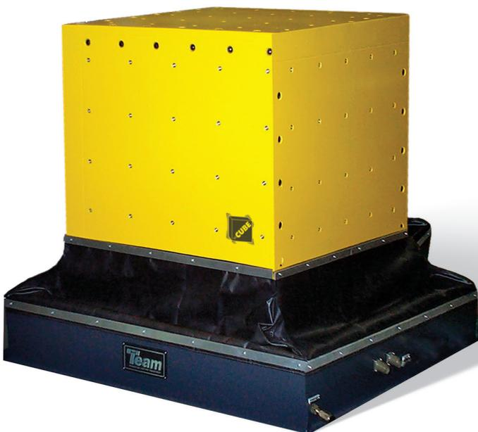
The CUBE™ simulates real-world vibration with complete, simultaneous control of the amplitude and phase of all 6 Degrees of Freedom. Offering simultaneous or sequential excitation of test articles in Sine, Random and Time Wave Form Replication, the CUBE™ sets the standard for multi-axis vibration testing.
