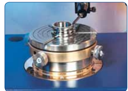
Gauge arm in horizontal attitude with orientation downward to measure top face
