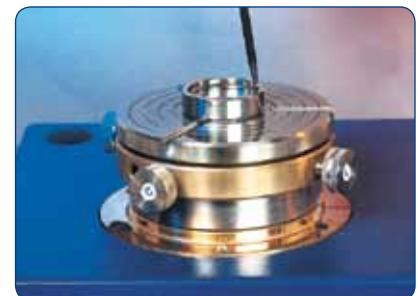
gauge arm in vertical attitude with orientation retracted to measure an inside diameter
