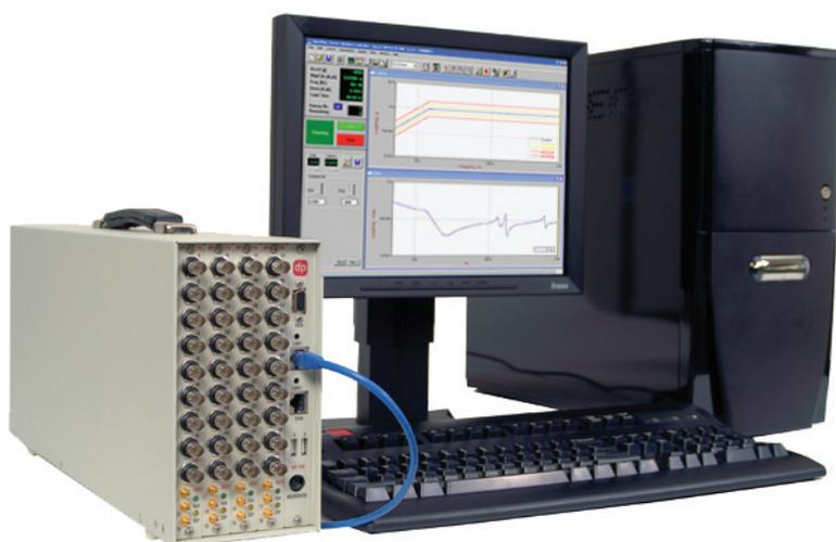
Software selectable single ended and differential inputs eliminate common mode noise associated with ground loop problems. TEDS support and ICP power are provided under software control.
