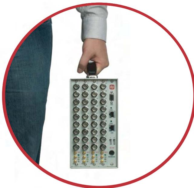
With its small size, light weight, and DC power option, the Mobilyzer is truly mobile. With up to 32 input channels, 8 output channels, and 8 tachometer channels, it is able to address large applications. Delivering a realtime rate of 49kHz, and over 120dB dynamic range, it is the analyzer that makes no compromises for being portable.
