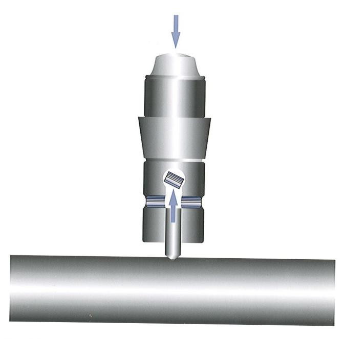
The ERNST calibrated pin system replaces the impact bar system giving a greater versatility and high accuracy. The indentations can be made very quickly even by an unskilled operator. The indentation can be read immediately, or at a later time by an inspector.
