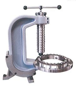
The static system allows load application via a lever on a clamp, particularly suitable for testing of castings.
