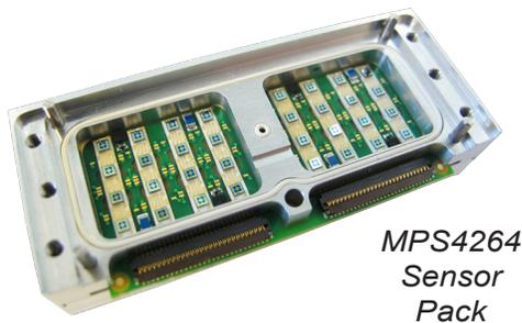
Along with the pressure sensors, all components in the measurement circuit are effected by temperature and drift over time. Scanivalve designed a patented architecture which continuously corrects for these changes over time, while the unit is scanning. This technique of "Dynamic Zero Correction" greatly improves the stability of the entire system over time and temperature. This is accomplished completely "behind the scenes," does not affect performance and requires nothing of the user.
