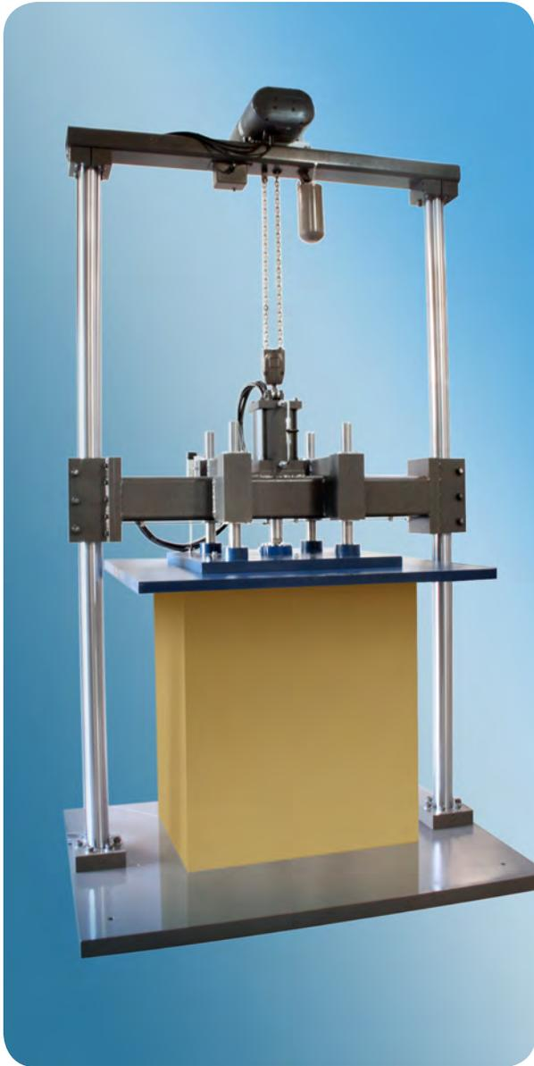
Severe compressive forces occur when packaged-products are stacked during transit or storage. To evaluate the performance of packages, components, and materials under such loads, Lansmont offers a full line of Compression Testers. Lansmont Compression Testers comply with industry standard package testing specifications including ASTM, ISTA, ISO, and MIL-STD.
