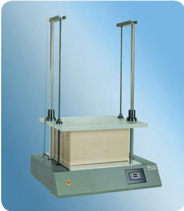
Severe compressive forces occur when packaged-products are stacked during transit or storage. To evaluate the performance of packages, components, and materials under such loads, Lansmont offers a full line of Compression Testers. Lansmont Compression Testers comply with industry standard package testing specifications including ASTM, ISTA, ISO, and MIL-STD.
